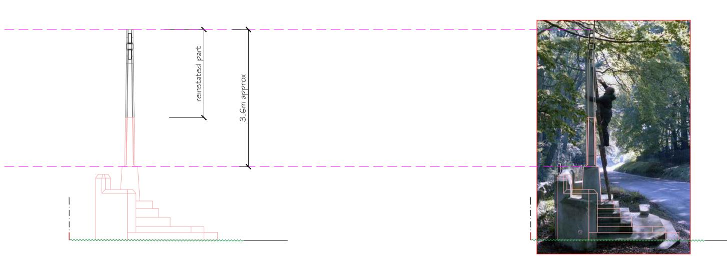
drawing of existing based on current site dimensions; as proposed based on limited photographs of original; stonework only to be carried out following detailed survey and to stonemasons design.
